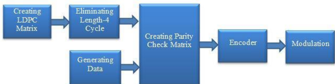
Fig. 3: Transmitter of LDPC system
